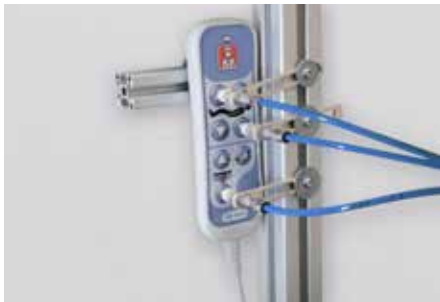
Resistance test on pendant
