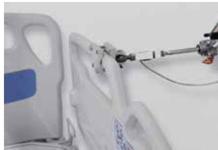
Push/Pull test on siderails
