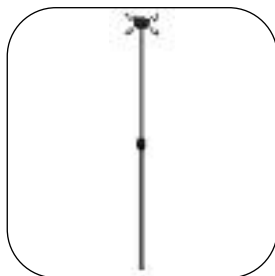
P158A Transfer Pole ..... Requires a P976H01 ISS Support Arm Mount. Mounts to main raceway only on Integris. Retracted position 32". Fully extended 57-1/4". Diameter to top pole 1/2". Diameter to outer pole 1".
